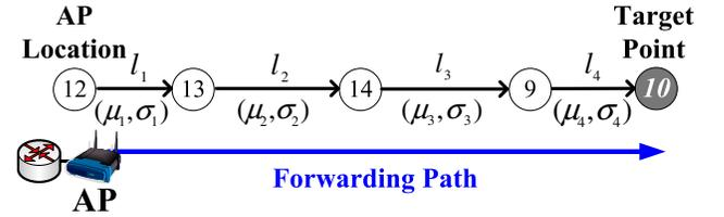
Figure 6. Packet Delay Model from AP to Target Point
