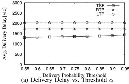
(a) Delivery Delay vs. Threshold  $\alpha$
