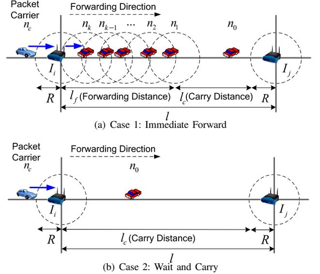
Figure 5. Link Delay Modeling for Road Segment
