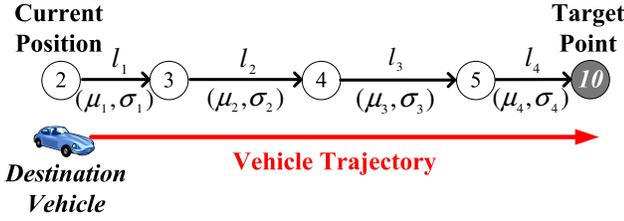
Figure 7. Vehicle Delay Model from Current Position to Target Point
