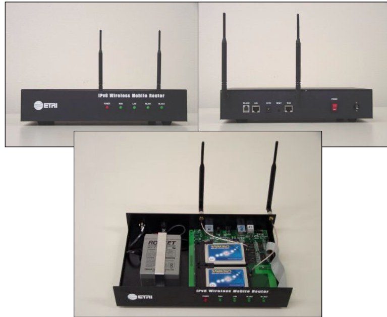
Fig. 8. IPv6 Wireless Mobile Router
