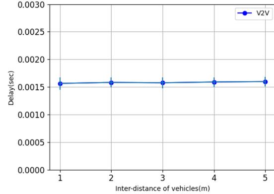
Fig. 5. Average Delay according to Distance between Vehicles design.
