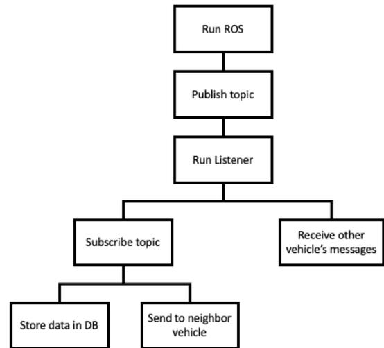
Fig. 3. Vehicular Web Client’s work-flow diagram.
